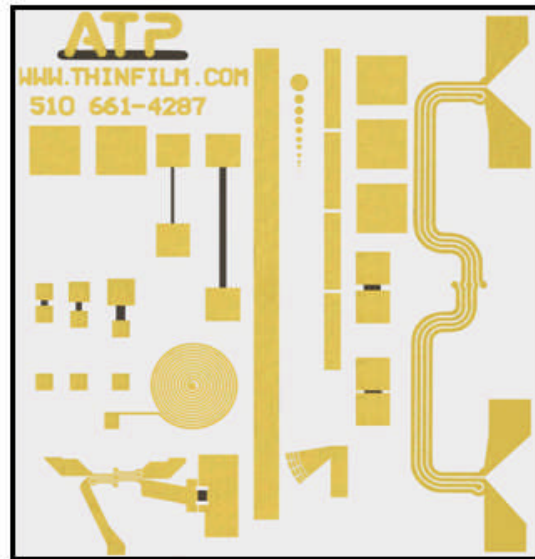
ATP1016, Material is 15 mil As-Fired Al 2 O 3
